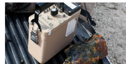
Slick rock sample with scintillometer, (Source: Anfield Energy)
